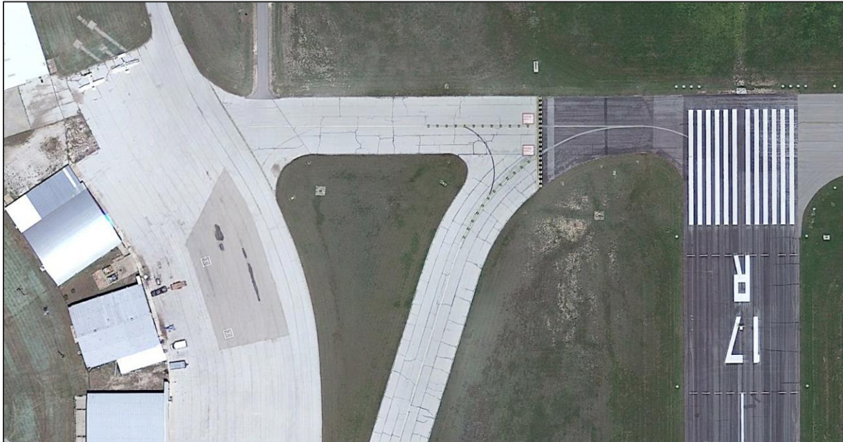
Figure 4-8 Taxiway R Intersection with Runway 17R/35L
